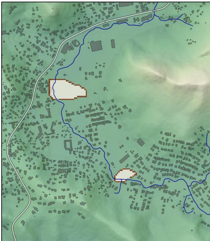
Figure 5.7. Configuration of four water buffers with varying size as half circular low dykes across the valley floor (indicated with arrows). Note that these are put in areas where the map does not show housing. This has not been checked with reality. From north to south the buffers have a size of 51200 and 15000 m 3 . Where the river crosses the barrier a maximum discharge of 15 m 3 /s has been assumed.
